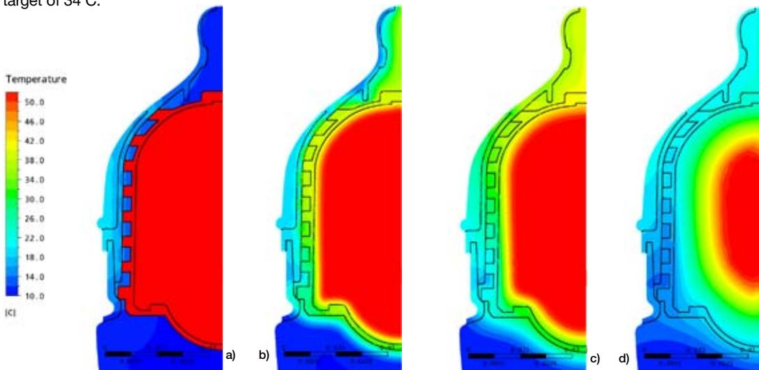
Temperature in prototype 3,  $k_{plug} = 10$  W/mK: **a)**  $t = 39.3$  s, **b)**  $t = 60$  s, **c)**  $t = 120$  s, **d)**  $t = 600$  s
