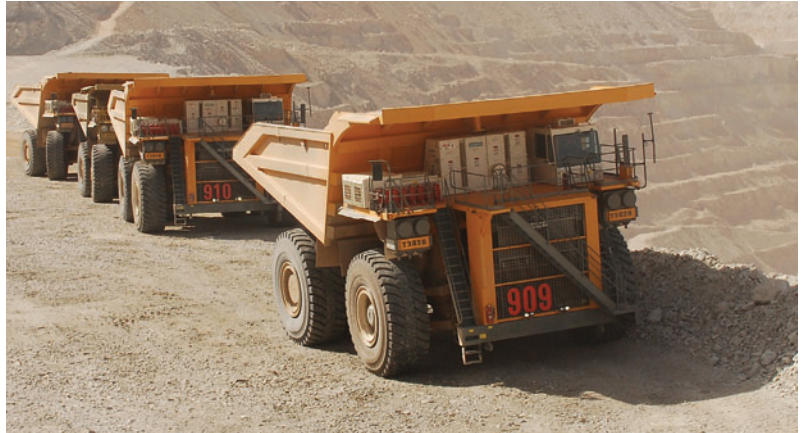
Ultra-class mining trucks are huge vehicles designed to transport heavy loads of raw materials over spiraling roads from the world's largest open-pit mines.
